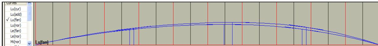
Above: Graph shows the difference in luff curve of the new sail. With the tack on the left and head on the right you can see how the luff curve has been biased towards the head.
